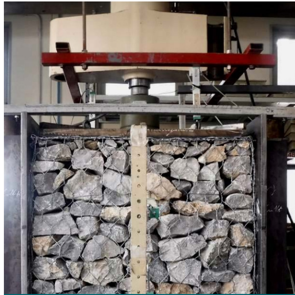
Full Scale Compressive Test
