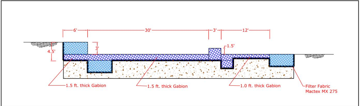
Typical long section through a drop structure
