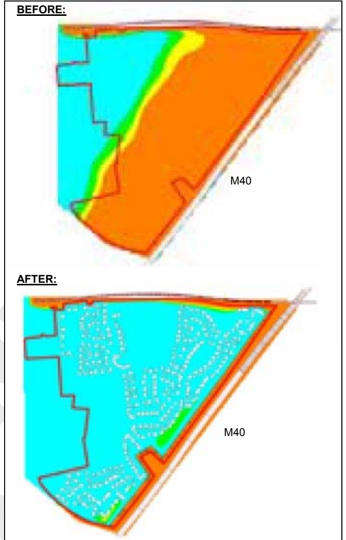
Before and after: the blue section shows how M-EC's bund proposal has created a viable area now under 55dB, which meets WHO guidelines.
