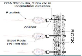
Drawing 1: Anchor connected with Paralink has been used in the construction
