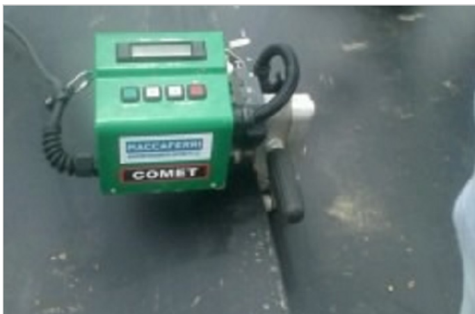
Photo 3: Joining of membranes by wedge welding machine
