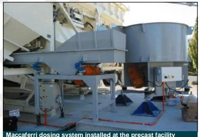
Maccaferri dosing system installed at the precast facility
