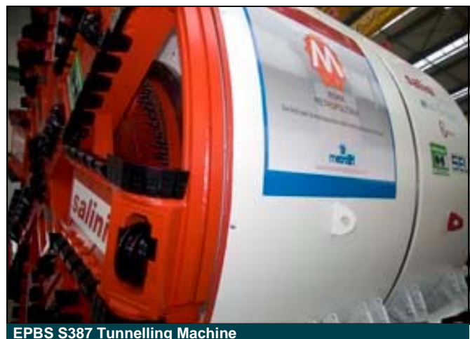
EPBS S387 Tunnelling Machine
