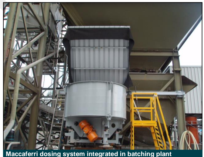
Maccaferri dosing system integrated in batching plant
