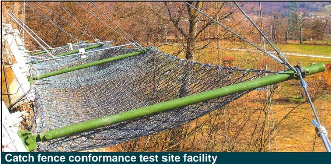
Catch fence conformance test site facility
