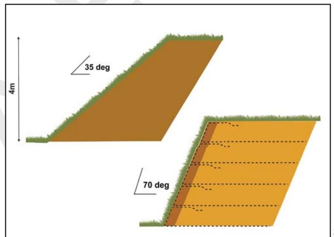
MacGrid<sup>®</sup> geogrid soil reinforcement safely steepens slopes
