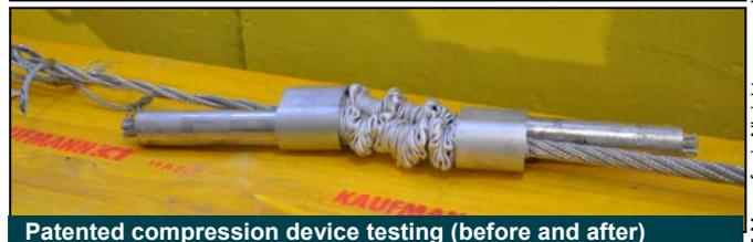
Patented compression device testing (before and after)
