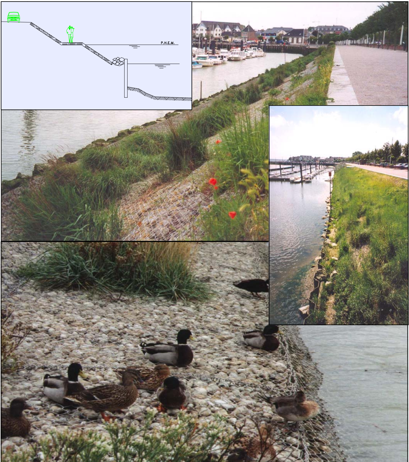
Typical project cross-section and completed project views
