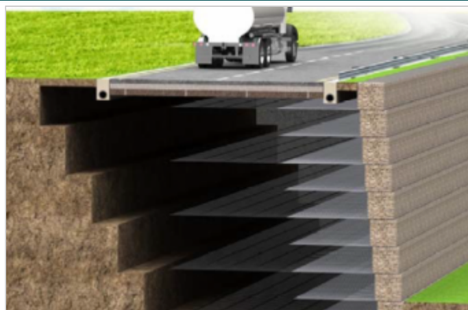
Typical schematic of hybrid Terramesh and ParaLink wall
