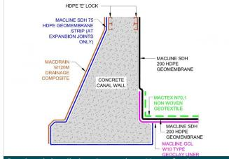
Sectional detail showing various Maccaferri geosynthetic products
