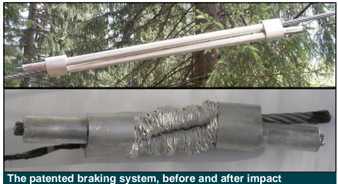
The patented braking system, before and after impact
