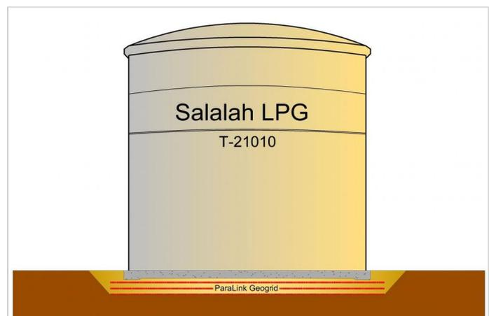
Sectional detail of tank, concrete foundation and ParaLink geogrid raft
