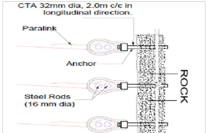
Drawing 1: Anchor connected with Paralink has been used in the construction
